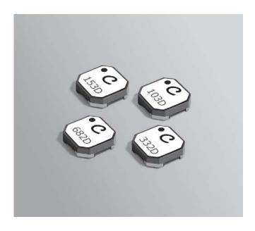
The LPD4012 coupled miniature shielded inductors are only 1,1 mm high and 4 mm square. Their excellent coupling coefficient (k ≥ 0.94) makes them ideal for use in SEPIC applications. In SEPIC topologies, the reguired inductance for each winding in a coupled inductor is half the value needed for two separate inductors. allowing selection of a part with lower DCR and higher current handling.
